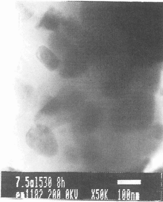
Fig.4a. TEM image of the glass-ceramics prepared from Glass A by the heat treatment at 530°C for 8h.
