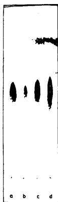
Fig. 1 Comparison of various cardiolipins on a thin-layer chromatogram. Development was in chloroform-methanol-water (70:25:4, v/v). Spots were revealed by charring after spraying with 10% H 2 SO 4 .
