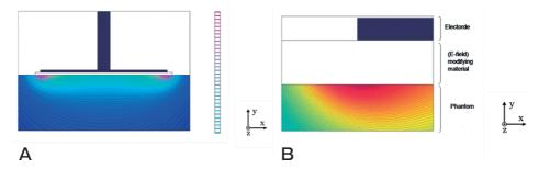
Fig. 4 SAR distribution when an E-field-modifying material is inserted between the flat plate electrode and the phantom; A, 1 mm thickness of E-field-modifying material (x-y plane at z = 0 mm); B, 2 mm thickness of E-field-modifying material (magnified view, x-y plane at z = 0 mm).
