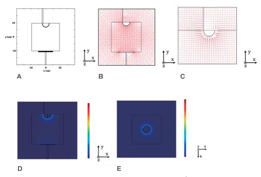
Fig. 7 SAR distribution when a hemispherical electrode is buried in the phantom; A, Arrangement of the hemispherical electrode; B, The vector of the electric field around the hemispherical electrode on the x-y plane at z = 0 cm; C, Magnified view on the x-y plane at z = 0 cm; D, SAR distribution on the x-y plane at z = 0 cm; E, SAR distribution on the z-x plane at y = 9.9 cm.
