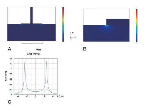
Fig. 3 SAR distribution when the flat plate electrode is placed on the phantom; A, SAR distribution on the x-y plane at z = 0 cm. Edge effects are seen around the end of the electrode; B, Magnified view of the end of the electrode; C, SAR profile along the x direction at the position of y = 9.9 cm, z = 0 cm.
