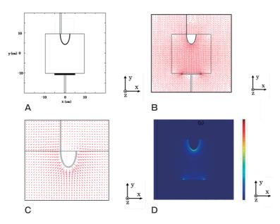
Fig. 6 SAR distribution when a hemi-ellipsoidal electrode is buried in the phantom; **A**, Arrangement of the hemi-ellipsoidal electrode; **B**, The vector of the electric field around the hemi-ellipsoidal electrode on the x-y plane at z = 0 cm; **C**, Magnified view on the x-y plane at z = 0 cm; **D**, SAR distribution on the x-y plane at z = 0 cm.
