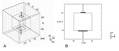
Fig. 1 Schematic diagram of simulation. A  $5 \times 5$  cm flat plate small electrode on the top, and a  $10 \times 10$  cm large electrode at the bottom of the cube-shaped muscle phantom,  $20 \times 20 \times 20$  cm. A, Orthographic projection; B, x-y view at z = 0.
