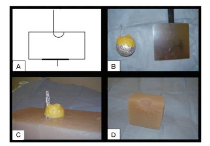
Fig. 2 Hemispherical electrode and agar phantom. A, Arrangement of electrodes and phantom; B, Hemispherical electrode (left) and external electrode (right); C, Hemispherical electrode buried in the top of the phantom; D, Bisecting plane of the phantom, which was measured with a thermographic recorder.
