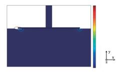
**Fig. 5** SAR distribution when the left edge of the flat plate electrode is covered with a polyethylene E-field-modifying material. The cross-sectional shape of the material is elliptical.
