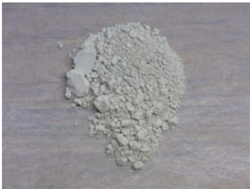
Fig. 8. Powder of the specimen obtained by wet-ball-milling 4.0 g of simulated waste slag powder with 300 ml distilled water for 20 hours once.
