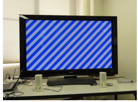
Figure 5: Stripe patterns in four directions are displayed on a large video screen.
