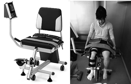
Fig. 2 Isoforce GT-330 (OG Giken) was used to measure maximum muscle strength of both legs during CKC exercise.
