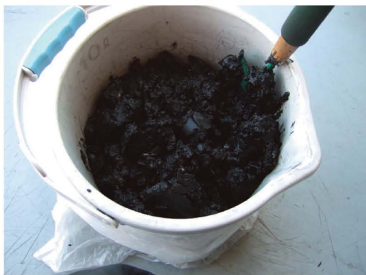
Fig. 1. Inorganic sludge discharged by the disposal of inorganic liquid waste in Environmental Management Center, Okayama University.
