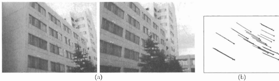
Figure 4: (a) Two images of a building and extracted feature points. (b) “Optical flow” consisting of segments connecting corresponding feature points (black dots correspond to the positions in the left image). The two endpoints can be identified with a point in a four-dimensional space.
