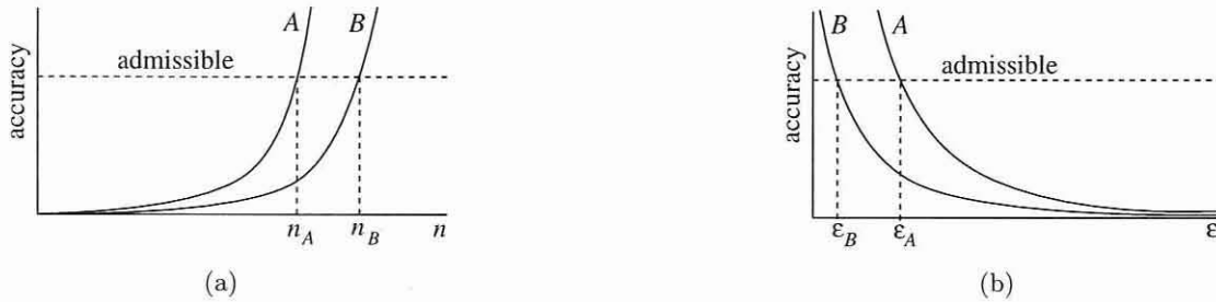
Figure 3: (a) For the standard statistical analysis, it is desired that the accuracy increases rapidly as the number of experiments n \rightarrow \infty , because admissible accuracy can be reached with a smaller number of experiments. (b) For geometric inference, it is desired that the accuracy increases rapidly as the noise level \varepsilon \rightarrow 0 , because larger data uncertainty can be tolerated for admissible accuracy.
