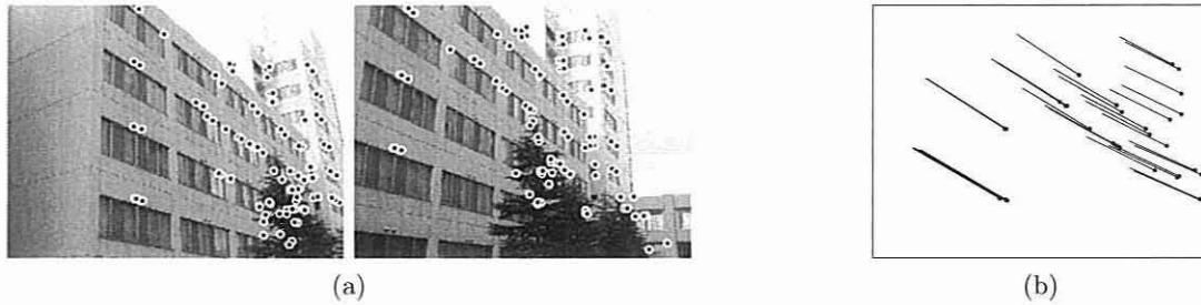
Figure 4: (a) Two images of a building and extracted feature points. (b) Optical flow consisting of segments connecting corresponding feature points (black dots correspond to the positions in the left image). The two endpoints can be identified with a point in a four-dimensional space.
