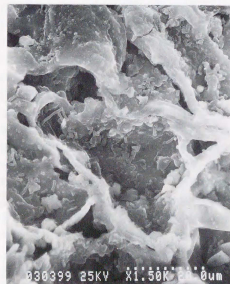
Fig. 15 SEM of the surface of an artificial stone incubated with E. coli No. 450 for 4 hrs.
