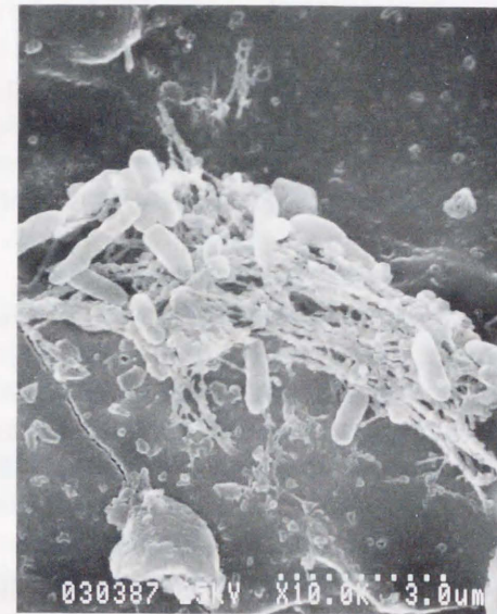
Fig. 14 SEM of the surface of an artificial stone incubated with P. aeruginosa No. 210 for 4 hrs.
