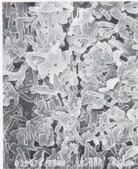
Fig. 4 SEM of bacterial colonization on a silicon disk surface 8hrs after contact with artificial urine containing 10^6 cfu/ml of E. coli No. 450.
