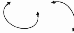
Figure 4: Judging if the edge segment covers more than the half of the ellipse.
