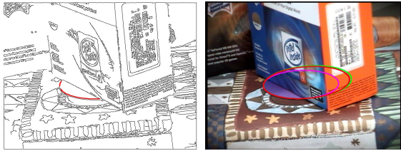
Figure 5: Left: Edge image containing a small elliptic edge segment (red). Right: Ellipses fitted to 155 edge points overlaid on the original image. From inner to outer are the ellipses computed by least squares (pink), Taubin method (blue), proposed method (red), and maximum likelihood (green). The proposed and Taubin method compute almost overlapping ellipses.
