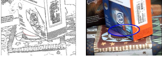
Figure 10: Left: Edge image of a circular object occluded to a large extent. Right: Ellipses fitted to the 148 edge points overlaid on the original image. The thin line is for LS, the white line is for Taubin's method, and the thick line is for the ML solution.
