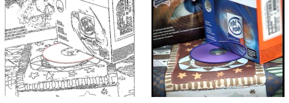
Figure 11: Left: Edge image of a circular object occluded to a small extent. Right: Ellipses fitted to the 414 edge points overlaid on the original image. The thin line is for LS, the white line is for Taubin's method, and the thick line is for the ML solution.
