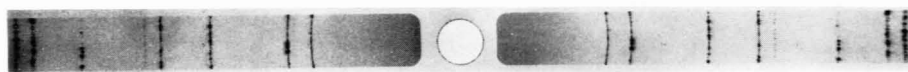
Photo. 2 Powder diffraction pattern of Al-6.8at% Zn alloy annealed at 125°C for 25 hours after quenching from 400°C into ice water.
