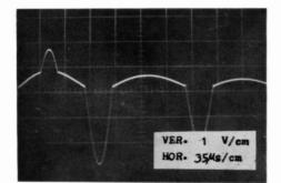
Fig. 14 Oscillograms of voltage corresponded to variation of water level in chamber surge tank.
