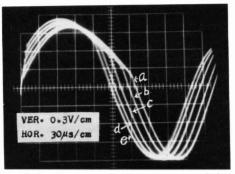
Fig. 10 Oscillograms of voltage corresponded to variation of water level in surge tank.
