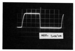
Fig. 3 Time-response of transistor switch.
