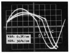
Fig. 11 Oscillograms of voltage corresponded to variation of water level in surge tank.
