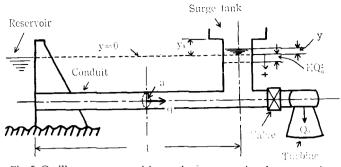
Fig. 5 Oscillatory system with varying cross-sectional surge tank.
