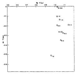
Fig. 2. Vector locus of the closed loop system.
