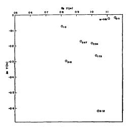
Fig. 6. Vector locus of the closed loop system : the input signal is complex and controlled system is proportional.
