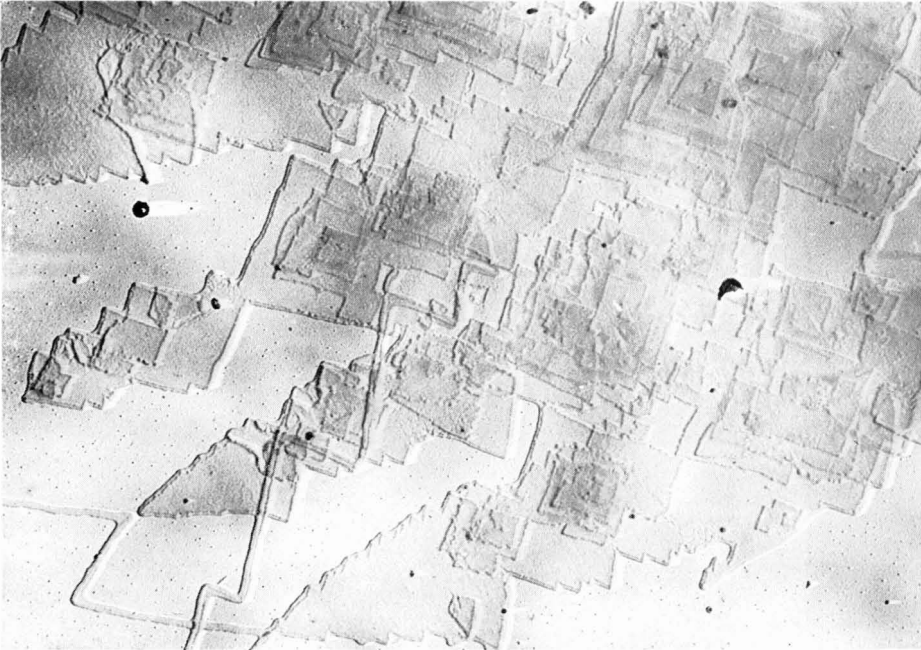
Fig. 2. Electron micrograph of dendritic crystals crystallized from solution. These crystals have a pronounced tendency for rapid growth to the diagonals. This growth mechanism is due to the way of screw dislocation. \times 10,000
