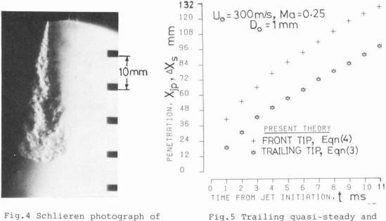
Fig.4 Schlieren photograph of hydrogen gas jet in still air
