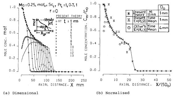
Fig.6 Axial distribution of hydrogen gas concentration on jet axis
