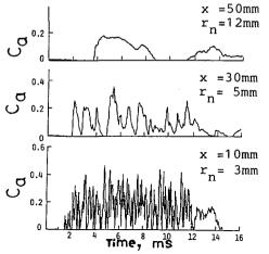
Fig.3 Transient hydrogen gas concentration near jet boundary
