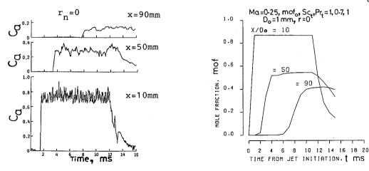
(a) Measurement-line mean(b) Prediction-point valueFig.2 Transient hydrogen gas concentration on jet axis locations
