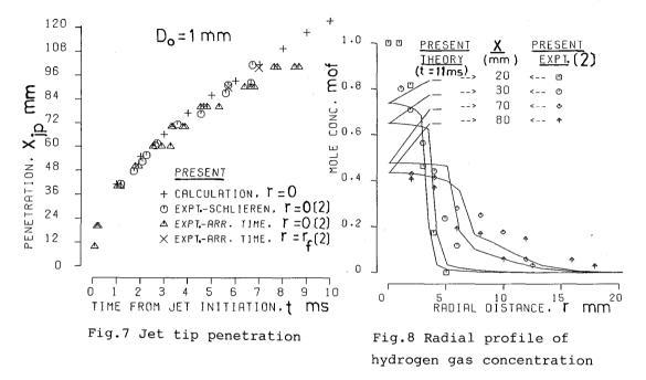
penetration measured by the method of arrival time at the two locations, r = 0 and  $r = r_f$ , of a given cross section. At x = 90, 100 mm, penetration measurements by photography and arrival time with  $r = r_f$  techniques seem to be in good agreement. The level of agreement between predicted and measured general trends of the jet tip penetration is reasonably good.
