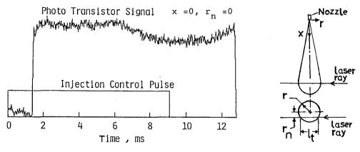
Fig.1 Signal at the nozzle exit
