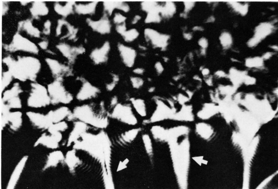
Fig. 3 Micrograph of polyethylene spherulites between crossed polaroids. ( \times 400 )
