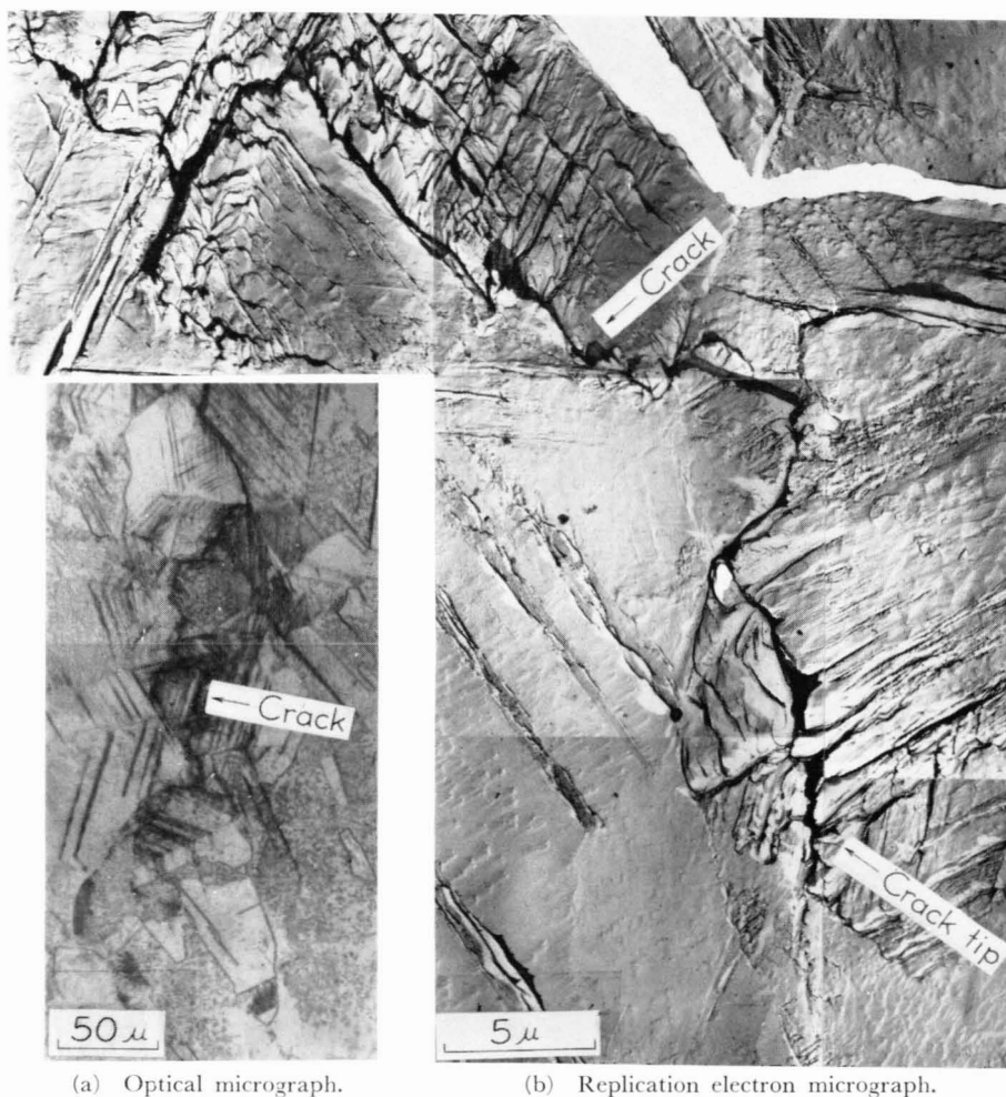
Fig. 6. Tip of propagating crack in pure copper specimen.
