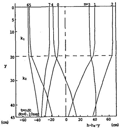
Fig. 21 Pore water pressure, Run 3 (calculated)
