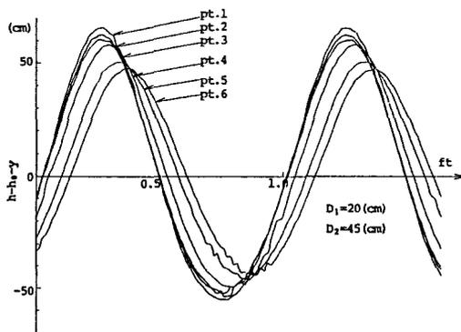
Fig.5 Pore water pressure, Run 3 (observed)
