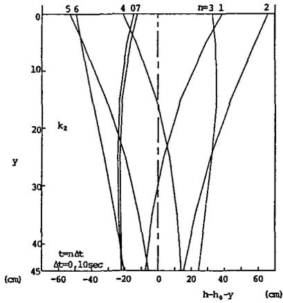
Fig. 19 Pore water pressure, Run 1 (calculated)
