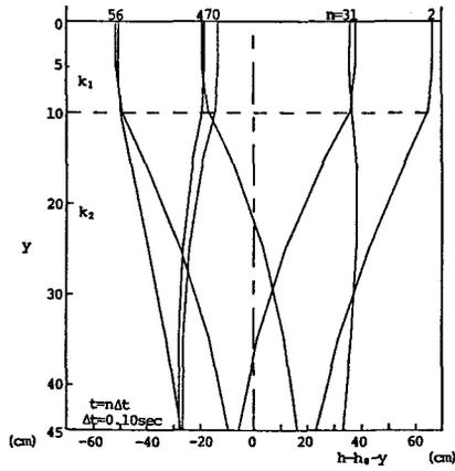
Fig. 20 Pore water pressure, Run 2 (calculated)
