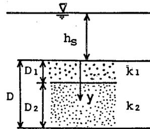
Fig.1 The definition sketch of the two-layered sand bed
