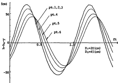
Fig.17 Pore water pressure, Run 3 (calculated)
