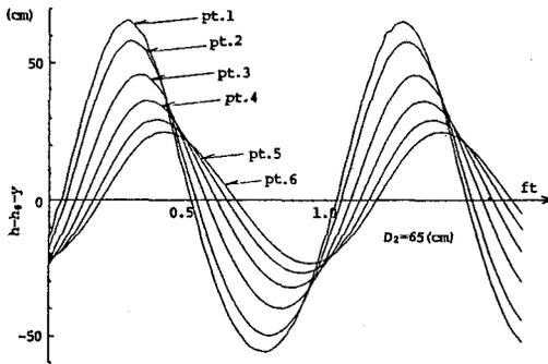
Fig.15 Pore water pressure, Run 1 (calculated)
