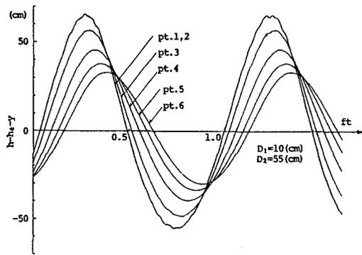
Fig.16 Pore water pressure, Run 2 (calculated)
