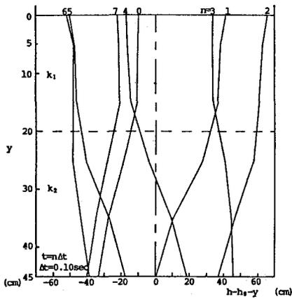
Fig. 9 Pore water pressure, Run 3 (observed)
