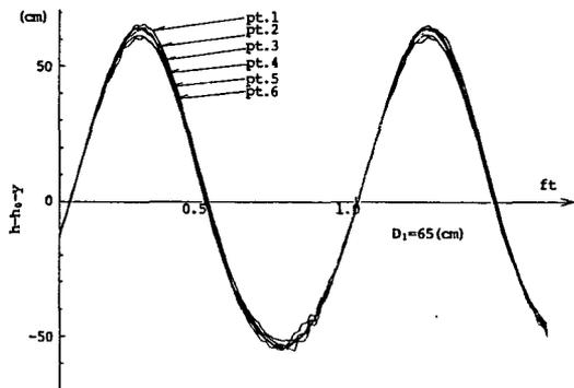
Fig.6 Pore water pressure, Run 4 (observed)
