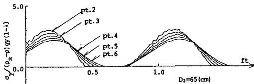
Fig. 23 Effective stress, Run 1 (calculated)
