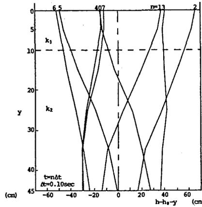
Fig. 8 Pore water pressure, Run 2 (observed)
