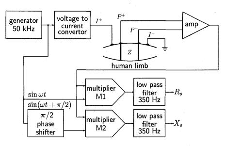
Figure 1 Block diagram of impedance measuring device.
