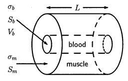
Figure 3 Parallel conductor model of human limb.
