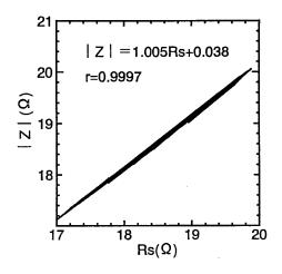
**Figure 2** Rissajous figure between |Z| and  $R_s$  during biodynamics.
