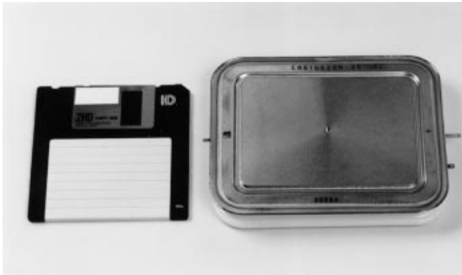
Fig. 1. Rectangular press-pack reverse-conducting IGBT rated at 2.5 kV and 1 kA.
