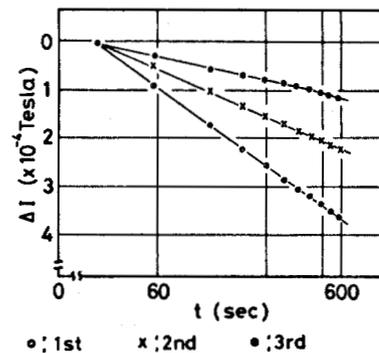
Fig. 5. After effect observed at the remanent state in cases of repeated measurements for a sample of a sort of samarium-cobalt magnet [5].
