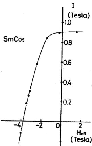
Fig. 3. Demagnetization curve I against effective field H in the case of applying 19 T for SmCo<sub>5</sub> magnet.
