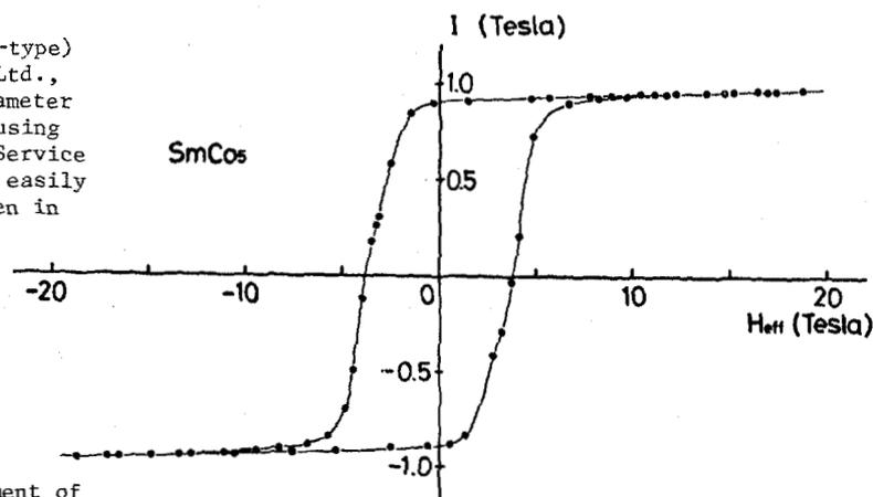
Fig. 1. Symmetric hysteresis loop of  $\text{SmCo}_5$  magnet measured at room temperature by applying maximum field of 19 T.
