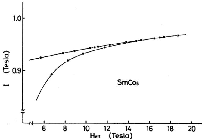
Fig. 2. The part of the magnetization curve approaching to the saturation and the decreasing part from the saturation magnetization of SmCo<sub>5</sub> magnet.
