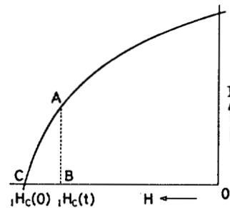
Fig. 4. Example of a magnetic field  $I_{H_c}(t)$  which becomes a coercive force owing to the existence of after effect.
