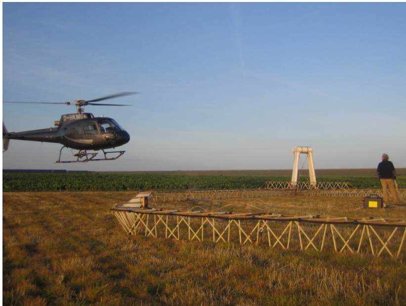
Fig. 10: SkyTEM System in operation – Netherland fieldwork (Set. 2009)
