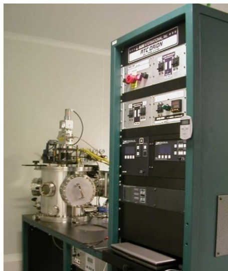
Figure 2.2 Aja International sputtering system.
