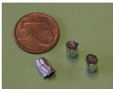
Figure 3. Tin capsules utilized to weight the coffee samples and introduce them in the elemental analyzer.
