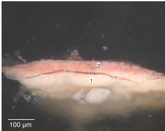
Figure D82. Cross section of the sample N1 - beige from the ground of Portão , viewed under reflected light.
