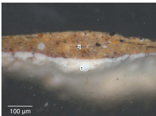
Figure D34. Cross section of sample G2 - brown from the ground of Cansada (cachopa de Capri) , viewed under reflected light.
