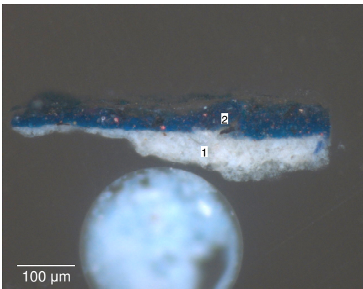
Figure D50. Cross section of sample I5 - dark blue from the skirt of Cecília , viewed under reflected light.
