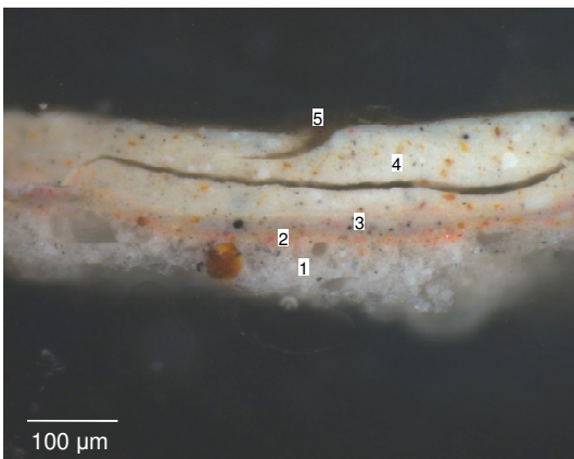
Figure D62. Cross section of the sample K5 - grey from canvas of Esperando o sucesso , viewed under reflected light.
