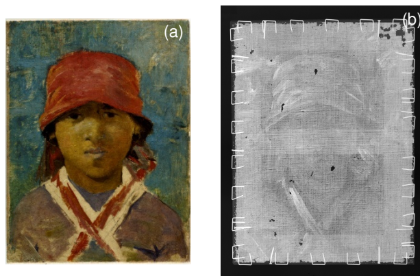
Figure 2.2 Rapariga de Anacapri (MNSR 200), 1882, oil on canvas, 18.5 x 13.8 cm: (a) photography; (b) X-radiography, where it is possible to see the wooden stretcher frame, the metal staple securing the fabric to a wooden stretcher and restoration areas (black areas). Photo and radiography: LCRJF.
