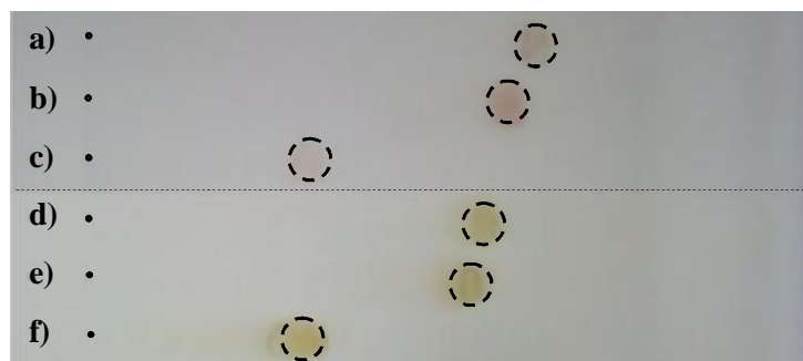
Figure 2.5 TLC of naringin (a), prunin (b), naringenin (c), rutin (d), isoquercetin (e) and quercetin (f).
