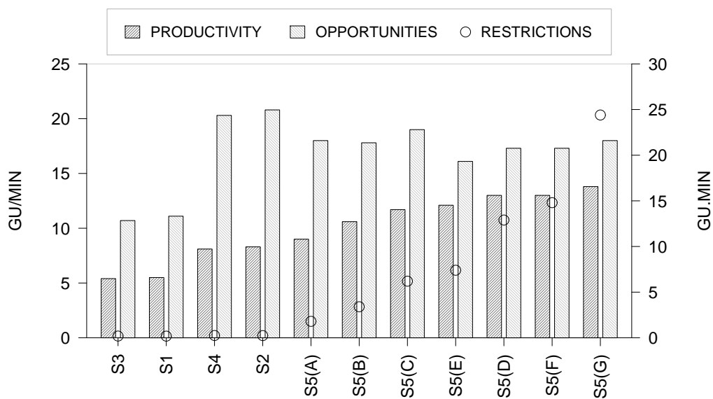
Figure 6.6: Comparison of productivity, opportunities, and restrictions. Sequences of tasks with greater productivity also impose much greater restrictions, and opportunities remain relatively constant.
