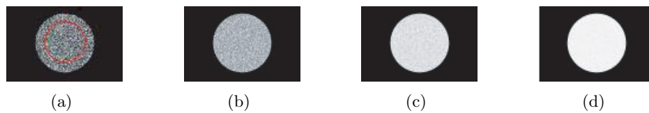
Figure 7.9: Central slice of the the images with an uniform circular area after adding Poisson noise. The images shown correspond to original with a) 10 counts per pixel, b) 100 counts per pixel c) 1000 counts per pixel and d) 10000 counts per pixel. In a) the Region of Interest that was used to analyze the images is shown.
