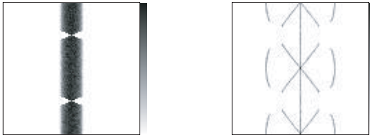
Figure 7.10: Images of the central slice of segment 0 sinograms of the Analytical Sphere Phantom (on the left) and of the Analytical Cross Phantom (on the right) after the addition of Poisson noise.
