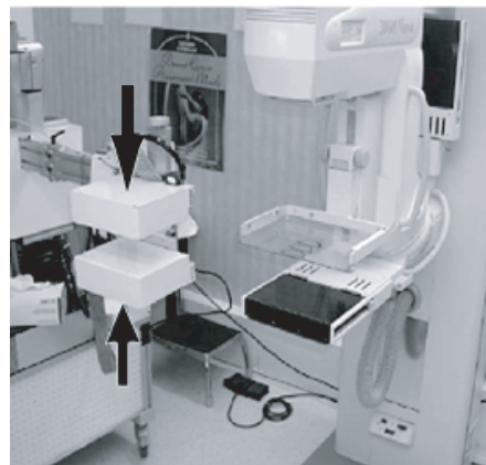
Figure 3.8: Image of the Duke University - Jefferson Laboratory PEM system positioned in a mammography unit. The PEM detectors are highlighted by black arrows. From [47].
