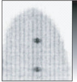
Figure 8.20: Uncorrected reconstructed image of the NCAT Breast phantom. The background region, that originally has constant activity, appears modulated due to the existence of regions of lower detection sensitivity in the scanner.
