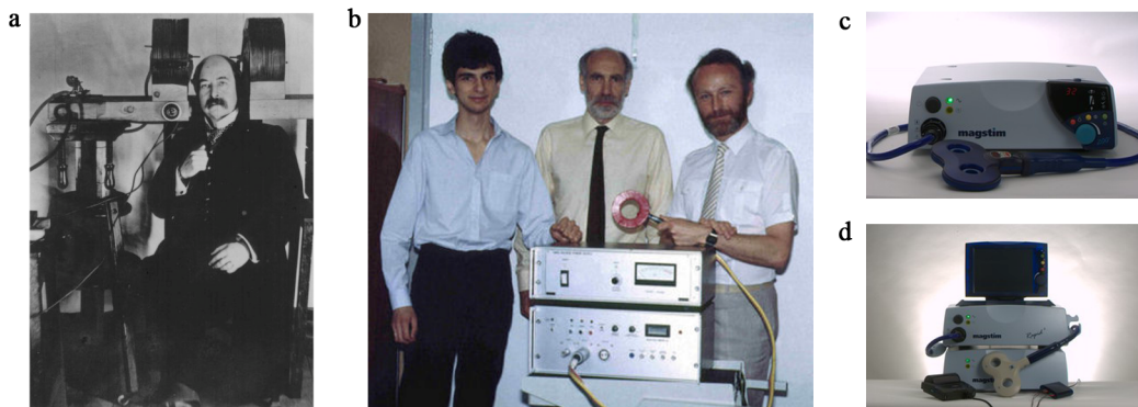
Figure 1.2.1.1: (a) One of the first devices used to investigate the induction of ‘magnetophosphenes’ by Silvanus P. Thompson in 1910; (b) The first magnetic stimulator developed by the Sheffield’s group, attached to a circular coil; (c) and (d) Modern-day magnetic stimulators: Magstim 200 stimulator and Magstim Rapid stimulator, respectively. Both stimulators are attached to a figure-8 coil (figures a and b taken from http://www.scholarpedia.org ; figure c and d taken from http://www.magstim.com ).
