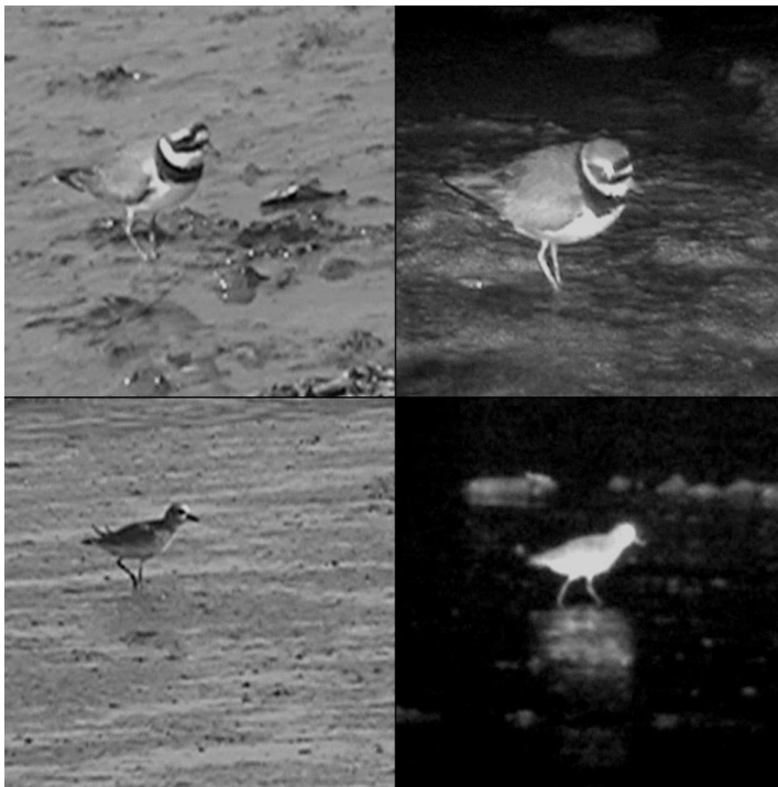
Figure 4.4. Captured frames from video recorded using our night vision system. A ringed plover at 25 m (top) and a grey plover at 85 m (bottom) during daylight (left) and at night (right).
