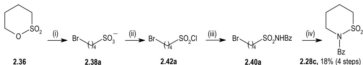
Scheme 2.20 Synthesis of the N -benzyl- \delta -sultam by cyclisation of the 4-bromo- N -benzylbutanesulfonamide. Reagents and conditions: (i) KBr, MeOH, reflux, 48 h; (ii) PCl 5 ; (iii) NH 2 Bz, DCM, -10 °C, 1 h; (iv) NaOH, TEA, MeOH, reflux.
