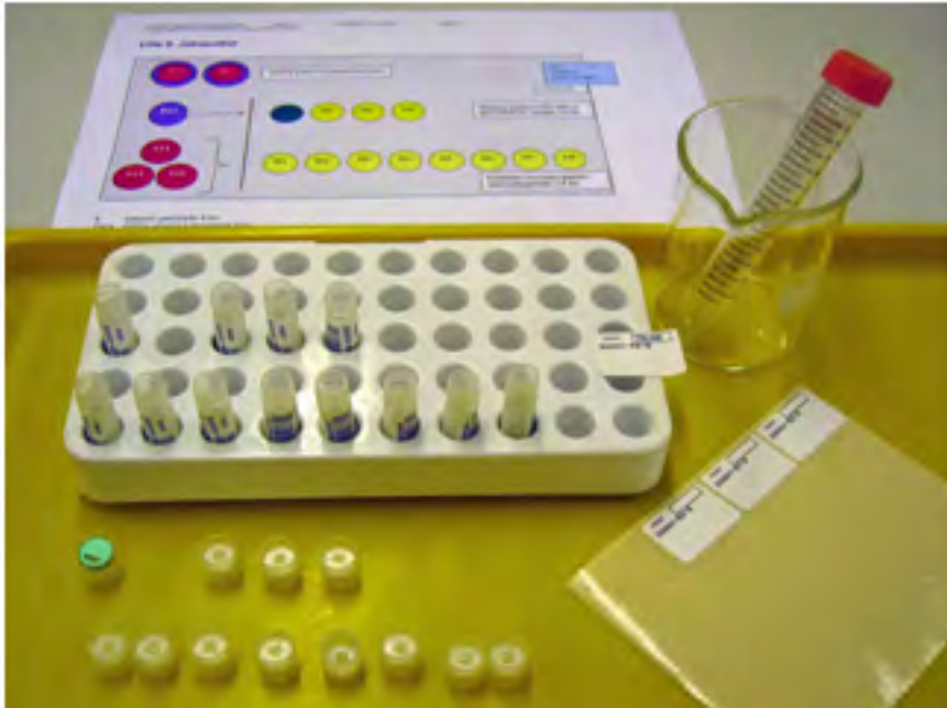
Figure 5.5.8. Caps of the storage tubes are removed in advance at the site of sample preparation. In the background is the pipetting scheme and in the foreground the label sheet in which the spare labels are left.
