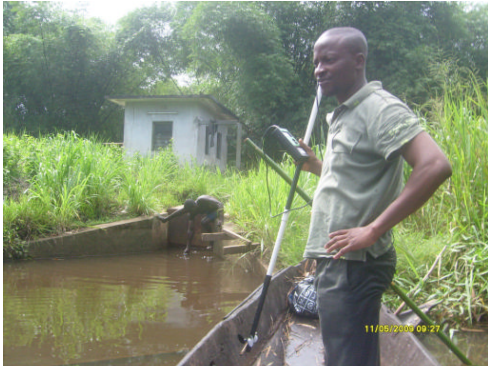
Plate 3.8: Geopacks Stream flow sensor with its pole and fan-like impeller
