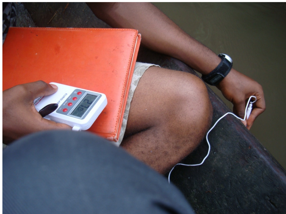
Plate 3.7: Eurolab digital thermometer with sensitive probe
