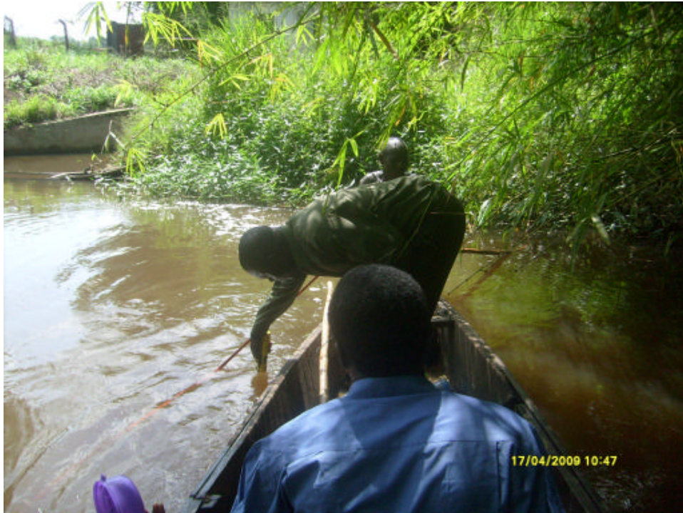
Plate 3.10: The Speedtech Portable Depth Sounder being used to measure depth
