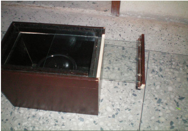
Figure 3: A picture showing the sliding glass cover with the box slightly open.
