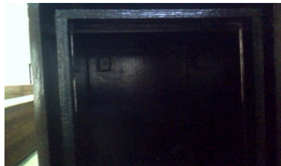
Figure 2: Picture showing the inner part of the box painted black to absorb heat.
