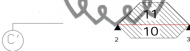
Gambar 6.3. Lebar Equivalen Balok Anak as C'(2 - 3) = E'''(2 - 3)
