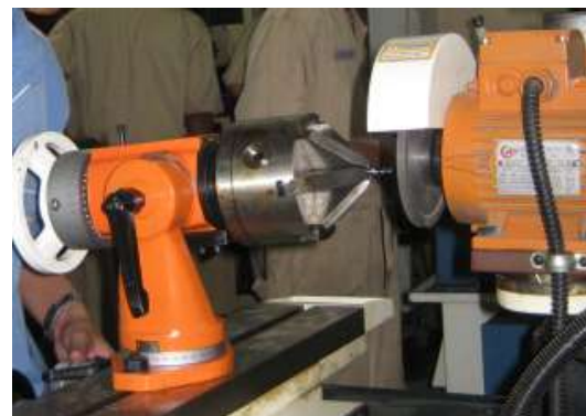
Gambar 12. Proses Penggerindaan Endmill Cutter
