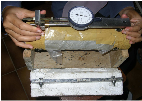
Fig. 1. Measurement of autogenous shrinkage using Demec Gauge
