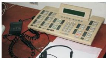
Gambar 54. PABX system Sumber: Ni Wayan Suwithi&Cecil Erwin Jr. Boham. 2008. Akomodasi Perhotelan , Jilid 1. Klaten : PT. Macanan Jaya Cemerlang.
