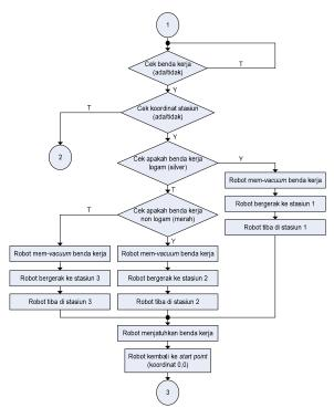
Gambar 6. Flowchart Kerja Robot Cartesian
