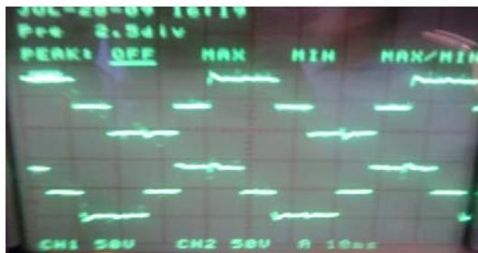
Gambar 4 Sinyal Output Inverter VB an VC
