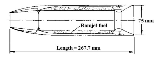
Fig. 4 SFRJ-assisted 75-mm gun launched projectile. 16
