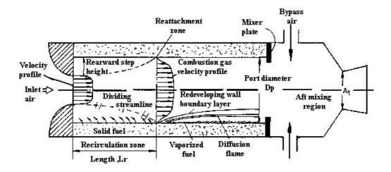
Fig. 2 Combustion chamber flow field in a solid fuel ramjet. 10, 11
