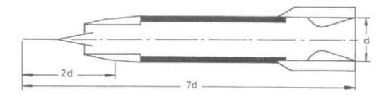
Fig. 6 Geometry of the SFRJ-assisted antitank missile.<sup>7</sup>
