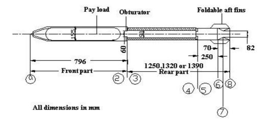
Fig. 1 Gun launched SFRJ-powered projectile.
