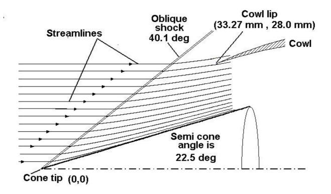
Fig. 9 Typical set of streamline pattern for M=1.6
