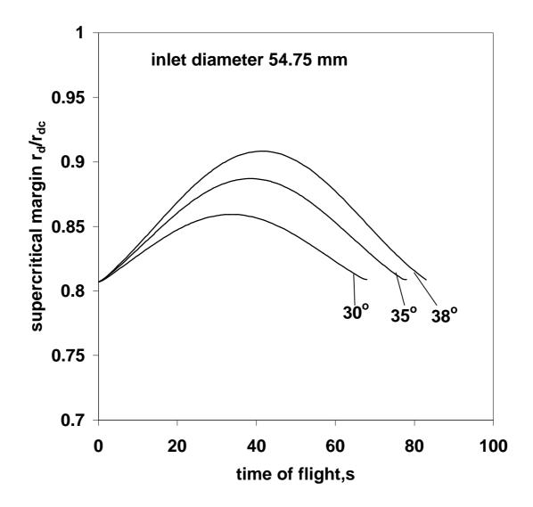
Fig. 12 Inlet operation under bypass control of inlet air. The fuel grain length is 1070 mm, the nose ogival slenderness ratio is 2.5, the annular gap is 5.0 mm, the constant A in the regression rate equation is  $8.5 \times 10^{-3}$ , and the throat diameter is 82 mm.
