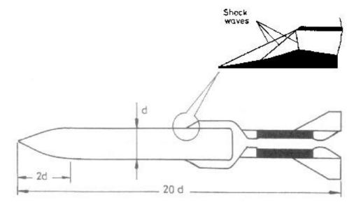
Fig. 7 Geometry of the high-speed air-to-air missile.  $^7$
