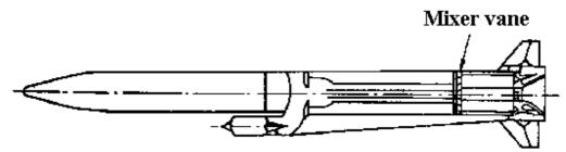
(a) Nonbypass with vane mixing device
