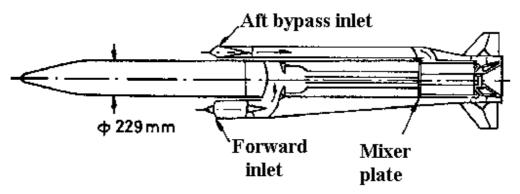
(b) Bypass with simple orifice mixing device
