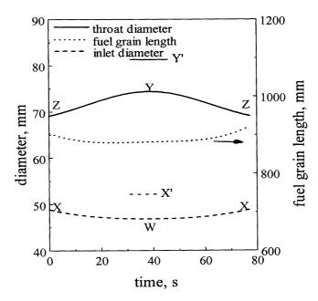
Fig. 8 Variation of fuel grain length, throat diameter, and inlet diameter. The launch angle is 35 deg, the nose ogival slenderness ratio is 2.5, the annular gap is 6.5 mm, and the constant A in the regression rate equation is  $8.5 \times 10^{-3}$ .
