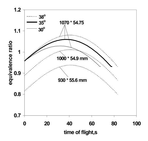
Fig. 11 Equivalence-ratio variations under bypass control of inlet air. The nose ogival ratio is 2.5, the annular gap is 5.0 mm, constant A in the regression rate equation is  $8.5 \times 10^{-3}$ , and the throat diameter is 82 mm.
