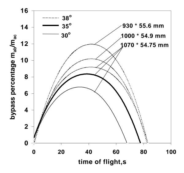
Fig. 10 Percentage variation of bypass ratio of inlet air. The nose ogival slenderness ratio is 2.5, the annular gap is 5.0 mm, the constant A in the regression rate equation is  $8.5 \times 10^{-3}$ , and the throat diameter is 82 mm
