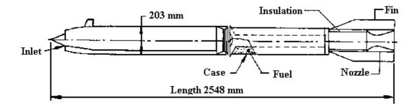
Fig. 5 SFRJ assisted 203-mm M110A-2 cannon launched projectile.<sup>16</sup>
