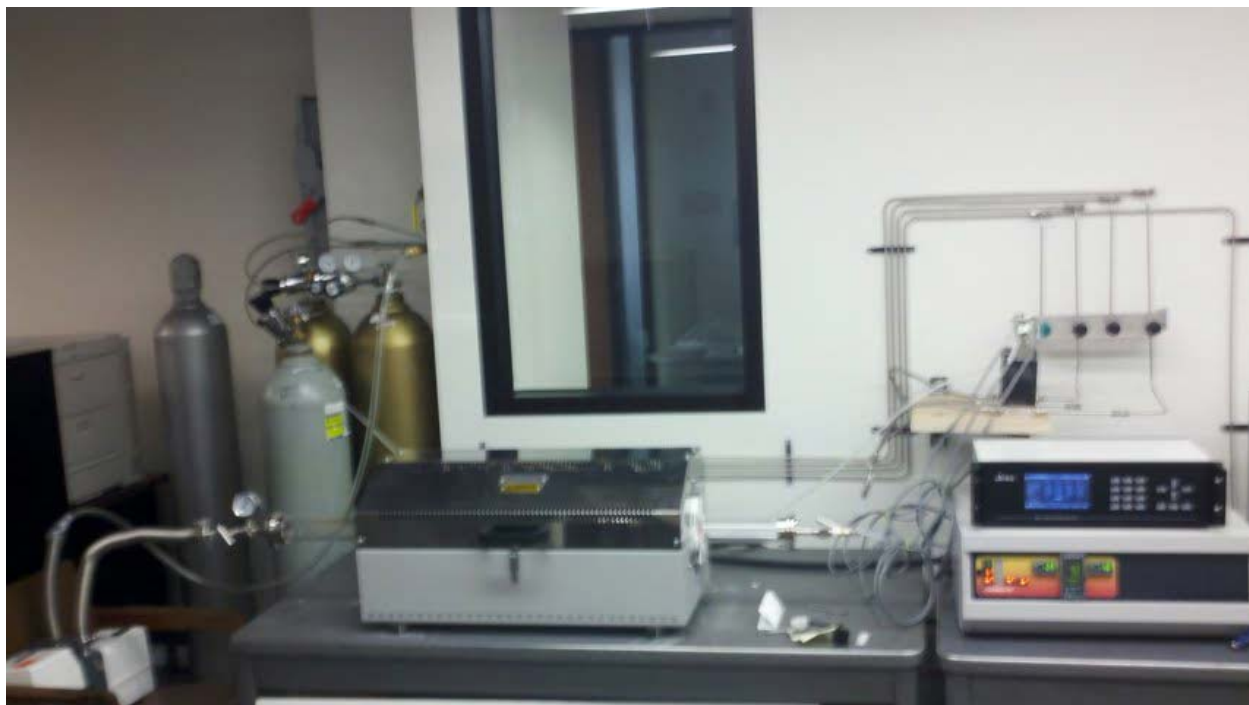
Figure 30. TCVD system based on a split-hinge Carbolite furnace retrofitted with Al 2 O 3 insulation to fit 50 cm quartz tubes. The system is interface to a computer using Labview (to the right of the visible furnace controller) with gas flow controlled using an MKS MFC system and flow controller. System is connect to roughing pump in this diagram although it can operate at atmospheric pressure by changing fittings.
