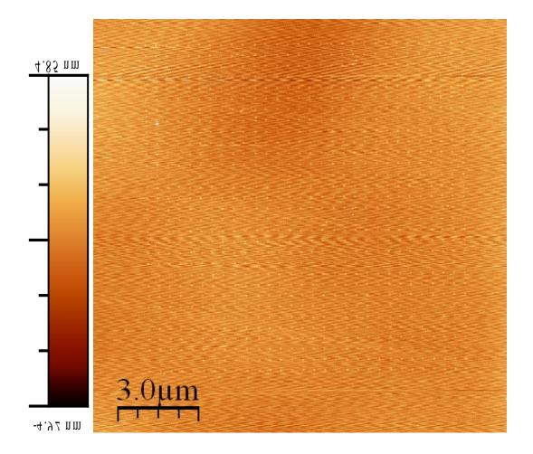
Figure 2.5 AFM image of FIB dot array pattern Si substrate. Dosage is  $3.0 \times 10^{15}$ /cm<sup>2</sup>, the voltage is 30 kV and the beam current is 1 pA.
