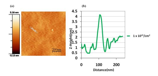
Figure 5.2 (a)AFM images of 1 x  $10^{15}$ /cm<sup>2</sup> dosage point arrays mills after SiGe alloy growth. (b) Profile data of the quantum dot. The sample's edge is roughly aligned along the <110> direction.
