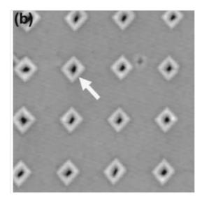
Figure 1.2 AFM 2 μm x 2 μm images of 20 nm Si<sub>0.7</sub>Ge<sub>0.3</sub> film grown at 550 °C and 0.9 Å/ s on a 7 nm Si buffer layer for patterned region within the FIB array. <sup>13</sup>
