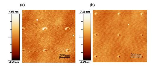
Figure 5.5 AFM images of 6 x  $10^{15}$ /cm<sup>2</sup> dosage point arrays mills after SiGe alloy growth. (a) SiGe alloy grown at 550 °C with total growth rate of 1 Å/s. (b) SiGe alloy grown at 450 °C with total growth rate of 0.5 Å/s. The sample's edge is roughly aligned along the <110> direction.
