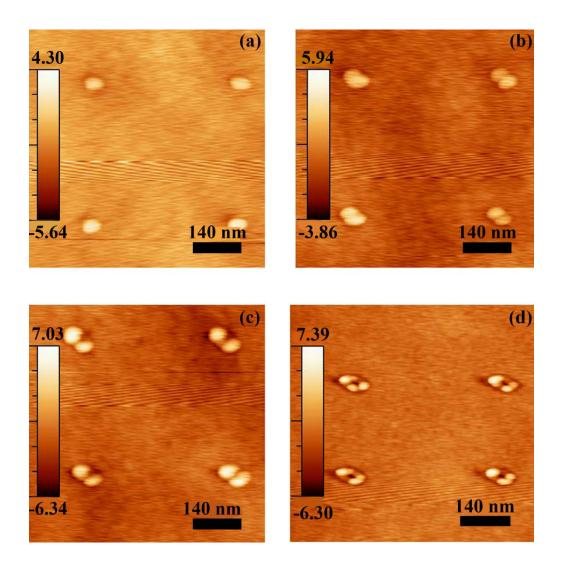
Figure 5.8 AFM 1x1  $\mu$ m image with edges roughly aligned along the <110> directions for films deposited on substrates patterned at single points using a 1 pA beam current. The 10nm Si<sub>0.7</sub>Ge<sub>0.3</sub> were grown on a 6.5nm Si buffer layer at 500°C and 1Å/s. Pattern dosages were (a) 0.5 x 10<sup>15</sup>/cm<sup>2</sup>. (b) 1 x 10<sup>15</sup>/cm<sup>2</sup>. (c) 3 x  $10^{15}/cm^{2}$ . (d) 6 x  $10^{15}/cm^{2}$ .
