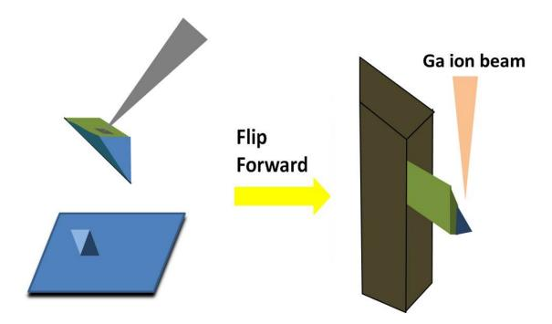
Figure 2.12 Plan view TEM samples preparation procedure.
