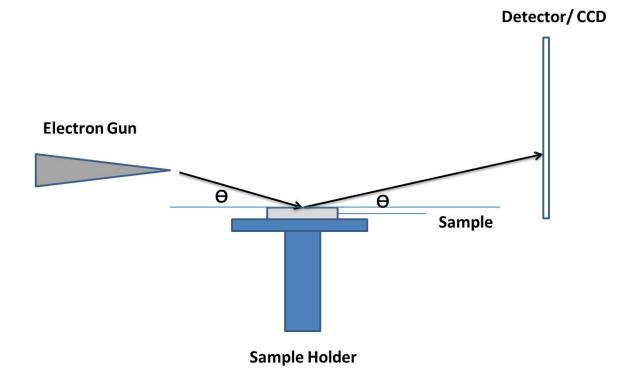
Figure 2.7 Schematic diagram of RHEED used in the research. .
