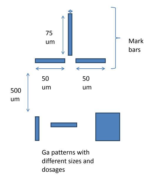
Figure 2.3 FIB pattern diagrammatic sketch (no to scale).
