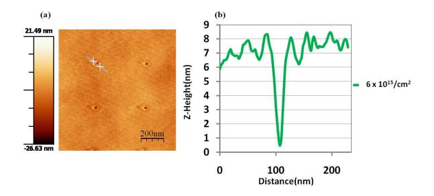
Figure 5.3 (a) AFM images of 6 x  $10^{15}$ /cm<sup>2</sup> dosage point arrays mills after SiGe alloy growth. (b) Profile data of the quantum dot. The sample's edge is roughly aligned along the <110> direction.
