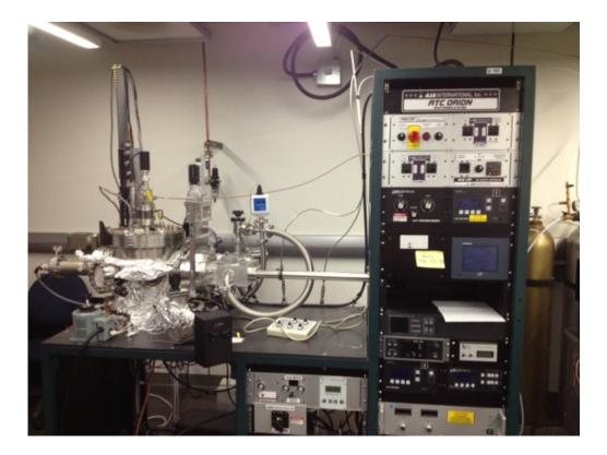
Figure 2.6 Magnetron Sputtering System used to grow all samples.
