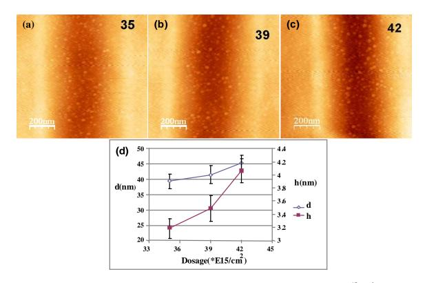
Figure 3.2 AFM image of trenches with different dosage after annealing: (a)  $35 \ge 10^{15}$ /cm<sup>2</sup>, (b)  $39 \ge 10^{15}$ /cm<sup>2</sup> and (c)  $42 \ge 10^{15}$ /cm<sup>2</sup> nm, (d) Ga nanodot diameter and height vs. dosage.
