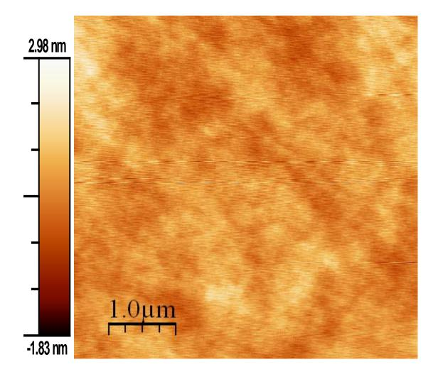
Figure 5.1 65 nm Si buffer layer grown at 500 °C.
