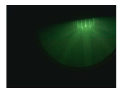
Figure 5.7 RHEED results for 10nm Si0.7Ge0.3 growth on 1.8 nm Si buffer layer at 550 °C and 1 Å/s.
