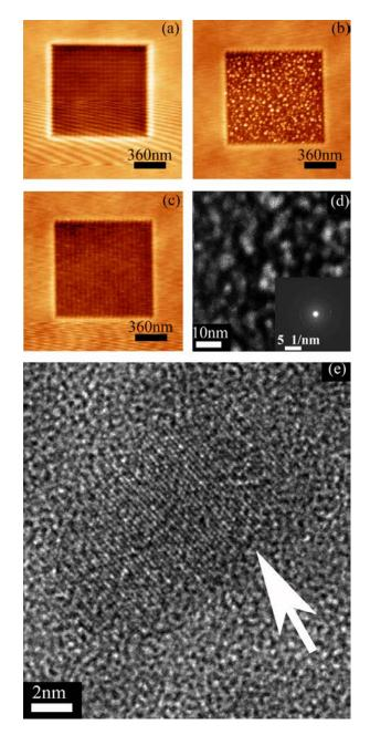
Figure 3.6 (a) AFM 2 x 2 μm image with edges roughly aligned along the <110> directions for Ga FIB pattern. Accelerating voltage was 30kv and the beam current was 5pA. The total ion dose was 2.9 x 10<sup>16</sup>
