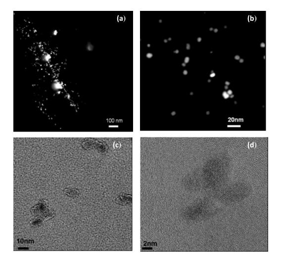
Figure 3.5 HAADF and HR-TEM images of Ga nanodots on amorphous silicon membrane: (a) HAADF of template, (b) HAADF at higher magnification, (c) HR-TEM of Ga nanodots and (d) HR-TEM of Ga nanodots at higher magnification.
