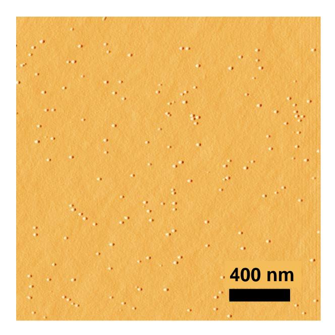
Figure 5.9 AFM of Ge quantum dots in un-patterned region.
