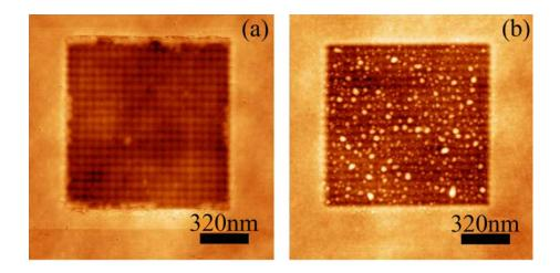
Figure 3.9 AFM 2 x 2  $\mu$ m image with edges roughly aligned along the <110> directions for Ga FIB pattern. Accelerating voltage was 10kv and the beam current was 5pA. Fluence was 2.9 x 10<sup>16</sup>/cm<sup>2</sup> for the 1 x 1  $\mu$ m patterned square area. (b) 1 x 1  $\mu$ m milled area after a after annealing for 1 hour at 600 °C.
