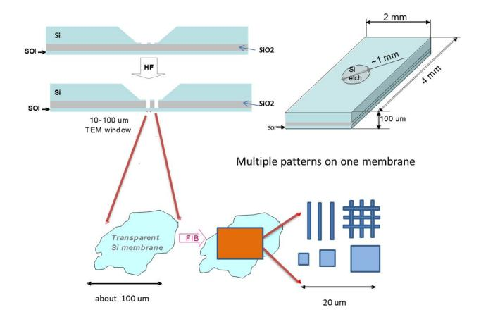
Figure 2.11 Fabrication Process of TEM samples.
