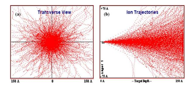
Figure 3.4 SRIM Monte Carlo simulation result of ions trajectories in Si with an accelerating voltage of 30 kV. Total number of ions is 1400. (a) Transverse view. (b) Ion trajectories.
