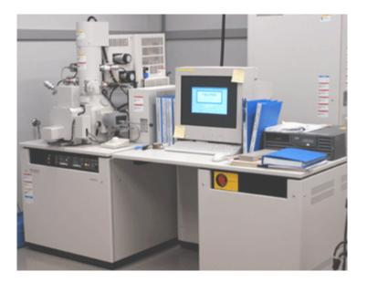
Figure 2.2 Focused Ion Beam System. 68
