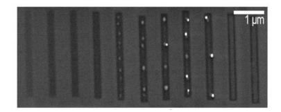
Figure 1.1 Ga nanodots on SiO2 surface fabricated by FIB with different dosages.<sup>29</sup>
