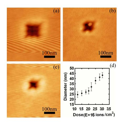
Figure 3.7 (a) AFM 1 x 1 μm image with edges roughly aligned along the <110> directions for Ga FIB pattern. Accelerating voltage was 30kv and the beam current was 5pA. Total dose was 2.9 x 10<sup>16</sup> ions/cm<sup>2</sup> for the 100 x 100 nm patterned square area. (b) 100 x 100 nm milled area after annealing for 1 hour at 600 °C. (c) 75 x 75 nm milled area after annealing for 1 hour at 600 °C. (d) Diameters of Ga nanoislands as a function of total ion dose.
