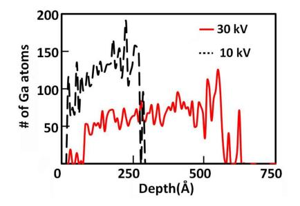
Figure 3.11 SRIM Monte Carlo simulation result of ions trajectories in Si with an accelerating voltage of 30 kV and 10 kV. Total number of ions is 1700.
