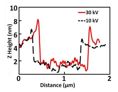
Figure 3.10 Depth profile (obtained from AFM scan) of 1 x 1  $\mu$ m patterned square area before annealing with different accelerating voltage. Total ion dose was 2.9 x 10<sup>16</sup> ions/cm<sup>2</sup> for the 1 x 1  $\mu$ m patterned square area.
