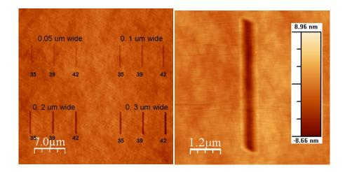
Figure 3.1 (a) overview AFM image of trench patterns before annealing. (b) Higher magnification of image of a single trench illustrating lack of topography in bottom of trenches before annealing. Image is of trench in lower left corner of Fig 3.1(a).
