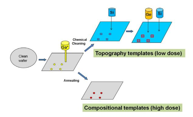
Figure 2.1. General experimental procedure in the FIB assisted nanostructure formation.
