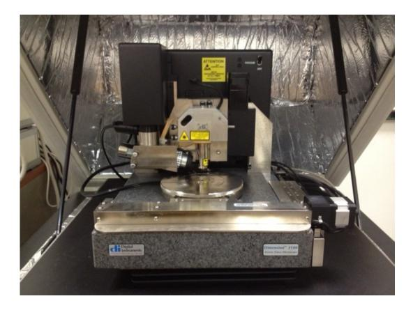
Figure 2.9 AFM used to characterize all samples.
