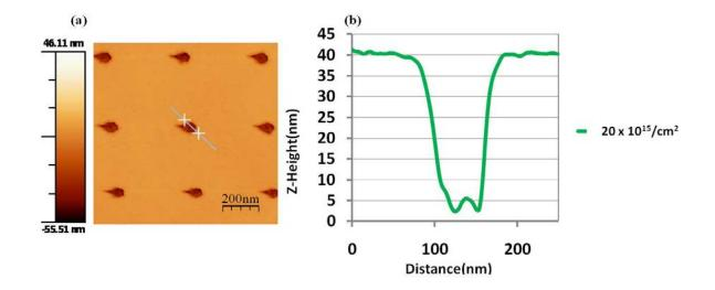
Figure 5.4 (a) AFM images of 20 x  $10^{15}$ /cm<sup>2</sup> dosage point arrays mills after SiGe alloy growth. (b) Profile data of the quantum dot. The sample's edge is roughly aligned along the <110> direction.
