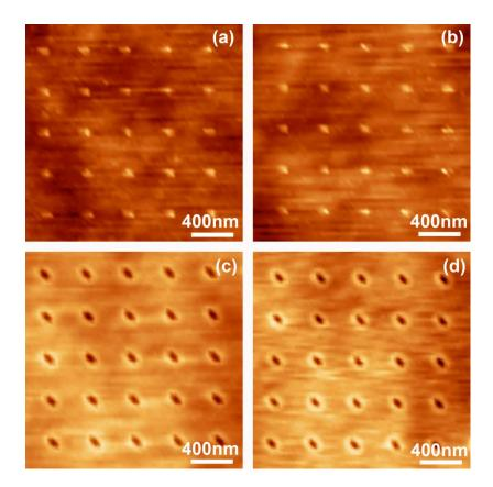
Figure 3.12 AFM images of (a) 1 pA beam current, 30 x 10<sup>15</sup>/cm<sup>2</sup> dosage point mills before and (b) after anneal. The z-scale for both images is 8.5 nm. (c) 10 pA beam current, 60 x 10<sup>15</sup>/cm<sup>2</sup> dosage point mills before and (d) after anneal. The z-scale for both images is 10.2 nm.
