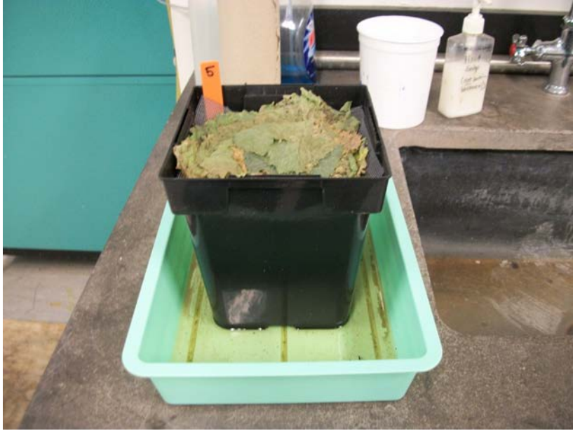
Figure 23. Photo showing a garlic mustard treated pot with tray from which water leachate samples were collected. Photo was taken seven days after the experiment began, so garlic mustard leaves are beginning to decompose.
