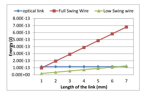
Figure 6: Comparisons on energy/power consumption of optical and electrical interconnects of different lengths [64, 71]
