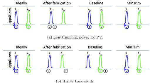
Figure 11: Two advantages of trimming  $\mu$ rings to a nearby wavelength.
