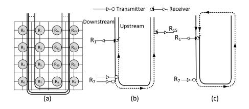
Figure 8: (a)Waveguide layout for a 16-node crossbar. (b) Single-Serpentine layout.(Data transmission:  $R_7 \rightarrow R_1$  and  $R_7 \rightarrow R_{15}$  via upstream and downstream channels)(c) Double-Serpentine layout.
