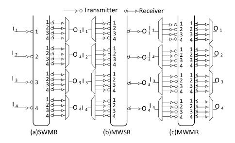
Figure 7: Crossbar microarchitectural design [4].
