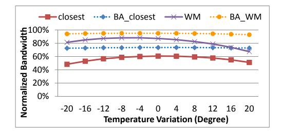
Figure 36: Network bandwidth Vs. temperature variations for CG-BandArb normalized to the bandwidth in the absence of PV and TF.
