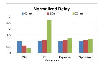
Figure 1: Gate, global wire(RC), global wire (repeater) and global wire (optimized+repeatered) delay [17]
