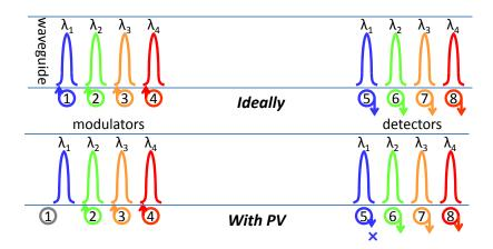
Figure 10: Bandwidth loss due to PV-drift.
