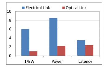
Figure 2: Relative latency, power and spatial bandwidth comparison chart for electrical and idealized optical link at 32nm technology node (in relative scale) [17]
