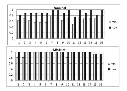
Figure 25: An example to show the maximum and minimum connection bandwidths of each node for "nominal" and MinTrim, respectively.
