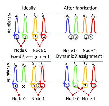
Figure 14: A case for flexible assignment between wavelengths and nodes.
