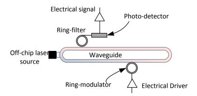
Figure 4: DWDM nanophotonic link.
