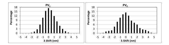
Figure 16: Distribution of wavelength shift for two sets of PV parameters in Table 3.
