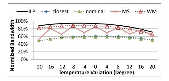
Figure 35: Network bandwidth Vs. temperature variations for local wavelength re-alignment normalized to the bandwidth in the absence of PV and TF.
