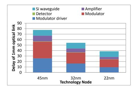
Figure 5: Delay breakdown for 1 mm optical link at different technology nodes [14]
