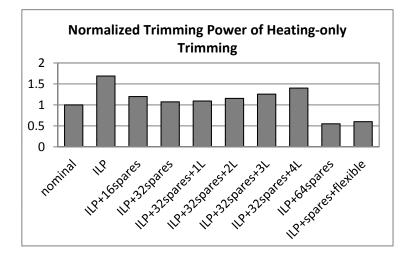
Figure 27: Normalized trimming power required by heating-only trimming.
