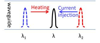
Figure 3: Power trimming method.  $\lambda$  indicates the nominal wavelength of  $\mu$ ring,  $\lambda_1$  and  $\lambda_2$  stands for the drifted resonant wavelength caused by PV or TF.
