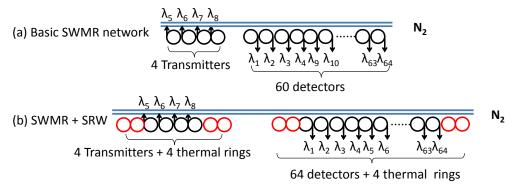
Figure 31: SWMR design of  $N_2$  with and without SRW [45].
