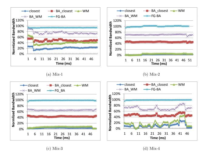
Figure 42: Normalized available bandwidth for communication with multi-programmed workloads.
