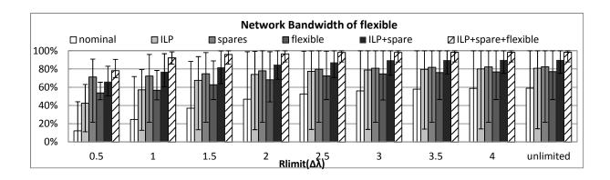
Figure 21: Bandwidth comparison between fix and flexible wavelength assignment.
