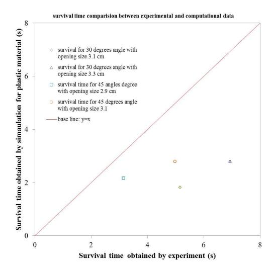
Figure 15: Comparison for survival time  $\tau$  of experimental and computational result for the plastic material.
