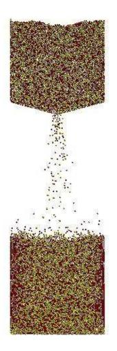
Figure 3: The configuration of the flowing particles in this hopper for angle 15° and opening size 4.5 cm by DEM simulation.
