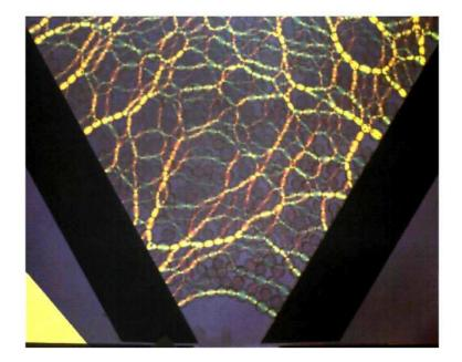
Figure 16: Image showing photoelastic particles between crossed polarizers. Evident is a strong force chain at the outlet which is supporting grains immediately above. Note: used by permission
