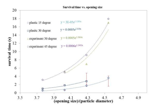
Figure 14: Comparison of experimental (green open triangle and pueple open circle) and computational (red open square and blue open diamond) result for the survival time.
