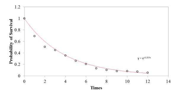
Figure 13: Probability that the flow of particles in the 2D hopper survives until time t obtained by DEM simulation. The red solid line is a fit to a decaying exponential with time constant  $\tau$ .
