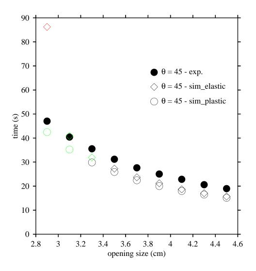
Figure 7: Comparison of experiment (solid bullets) and computational results of both elastic material (open diamond) and plastic material (open circle) for the 45° hopper's empty time. The different colors stand for different numbers of times of jams during the discharge process for both the elastic and the plastic materials of the computational data.
