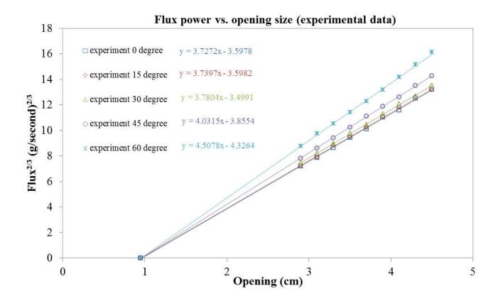
Figure 10: The experimental results for the hopper mass flux.
