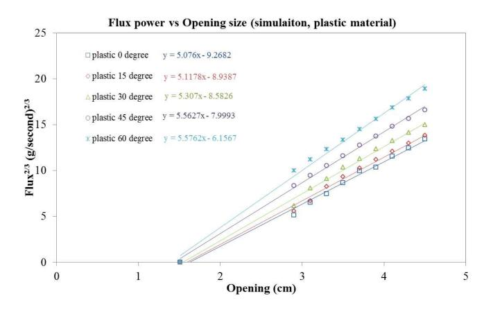
Figure 11: The computational results for plastic material for the hopper mass flux.
