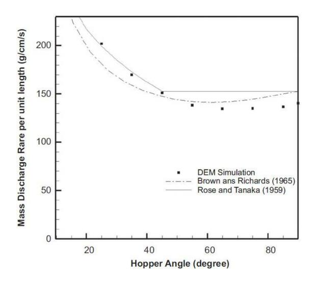
Figure 1: DEM mass discharge rate plotted against hopper angle [1]. The correlations by Brown and Richards and Tanaka are also plotted.
