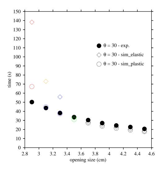
Figure 6: Comparison of experiment (solid bullets) and computational results of both elastic material (open diamond) and plastic material (open circle) for the 30° hopper's empty time. The different colors stand for different numbers of times of jams during the discharge process for both the elastic and the plastic materials of the computational data.
