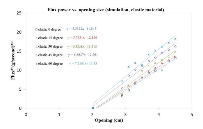
Figure 12: The computational results for elastic material for the hopper mass flux.
