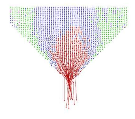
Figure 19: Velocity profile for the 45 degree hopper by DEM simulation
