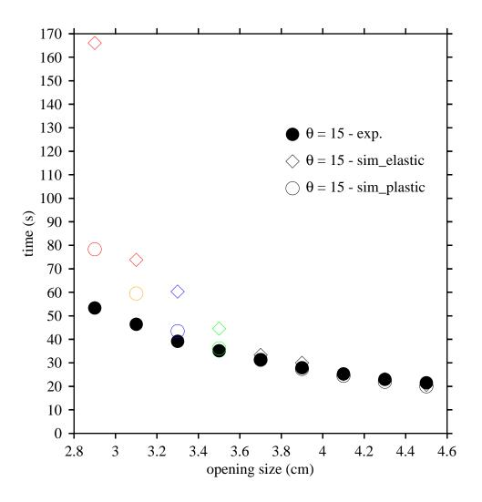
Figure 5: Comparison of experiment (solid bullets) and computational results of both elastic material (open diamond) and plastic material (open circle) for the 15° hopper's empty time. The different colors stand for different numbers of times of jams during the discharge process for both the elastic and the plastic materials of the computational data.
