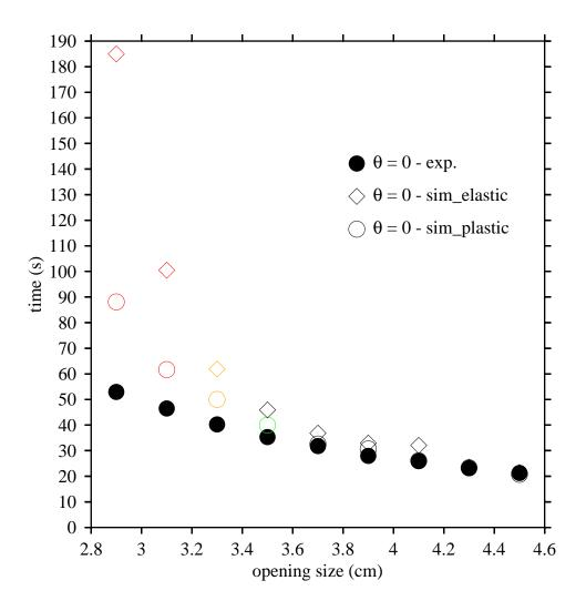
Figure 4: Comparison of experiment (solid bullets) and computational results of both elastic material (open diamond) and plastic material (open circle) for the 0 degree hopper's empty time. The different colors stand for different numbers of times of jams during the discharge process for both the elastic and the plastic materials of the computational data.
