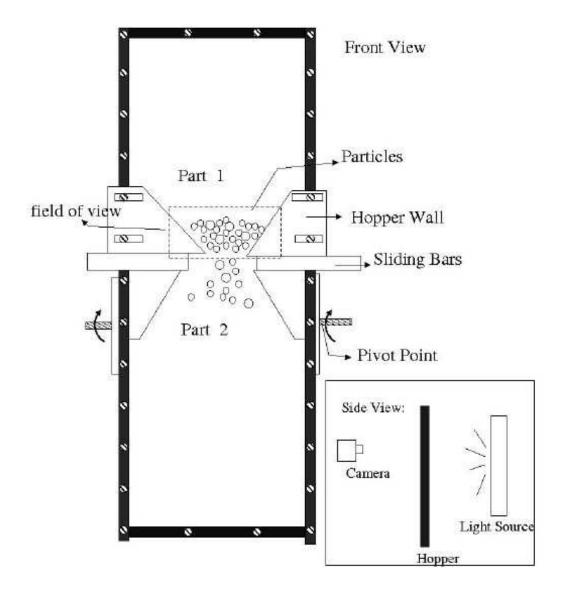
Figure 2: The schematic of hopper (used by permission)
