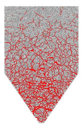
Figure 17: Particle normal stress profile for the 60 degree hopper by DEM simulation
