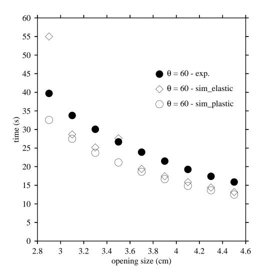
Figure 8: Comparison of experiment (solid bullets) and computational results of both elastic material (open diamond) and plastic material (open circle) for the 60° hopper's empty time. For 60 ° hoppers with different opening size, all the bullets are black, which stands for that no more than 5 times of jams happened in the simulation for both elastic and plastic materials.
