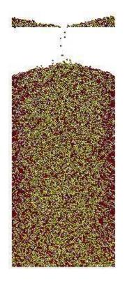
Figure 9: The configuration of the flowing particles in this hopper for 0 degree angle by DEM simulation when the hopper is nearly empty.
