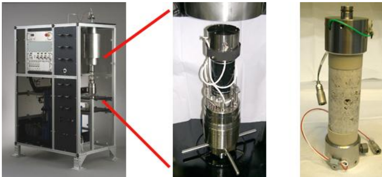
Figure 1: Left: NER Autolab 1500 Center: Sonic velocity core holder assembly Right: Resistivity heads with Limestone core.
